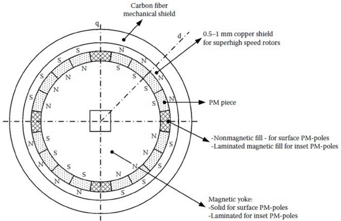
FIGURE Four-pole surface permanent magnet (PM) and inset PM pole rotor configurations.
