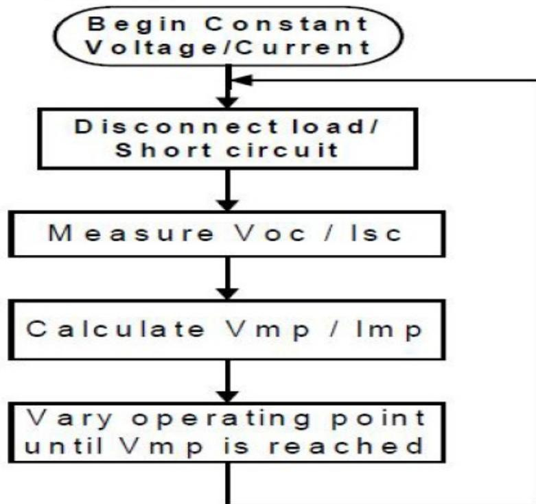
Figure Constant voltage/current algorithm flowchart
