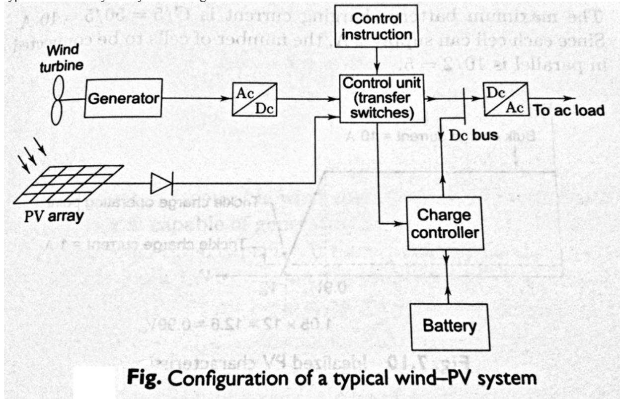
The ac output of the wind generator feeds a rectifier which is connected in parallel to PV array through a controller to a dc bus. The dc bus also serves as a connection point for the battery through a charge controller. The blocking diode protects the PV array from voltage spikes and prevents the flow of current in the reverse direction at low irradiation. The controller decides the connection of the generating system/battery supply, or its charging, in specific situations and requirements.
