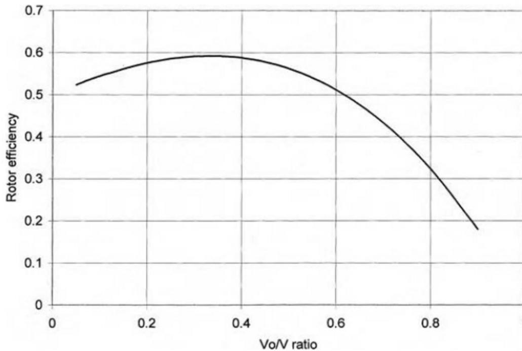
**Rotor efficiency vs.  $V_o/V$  ratio has a single maximum.**
