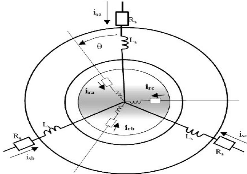
Figure : Induction machine's schematic illustration
