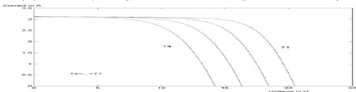
Below Figure shows the variation of PV current and voltages at different insolation levels. From Figs. 5 and 6, it can be seen that the I V characteristics of solar cells at a given insolation and temperature consist of a constant voltage segment and a constant-current segment. The current is limited, as the cell is short-circuited. The maximum power condition occurs at the knee of the characteristic where the two segments meet.
