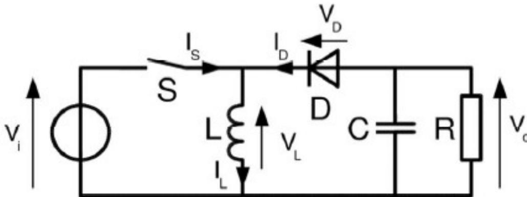
Fig 14 Buck Boost Converter
