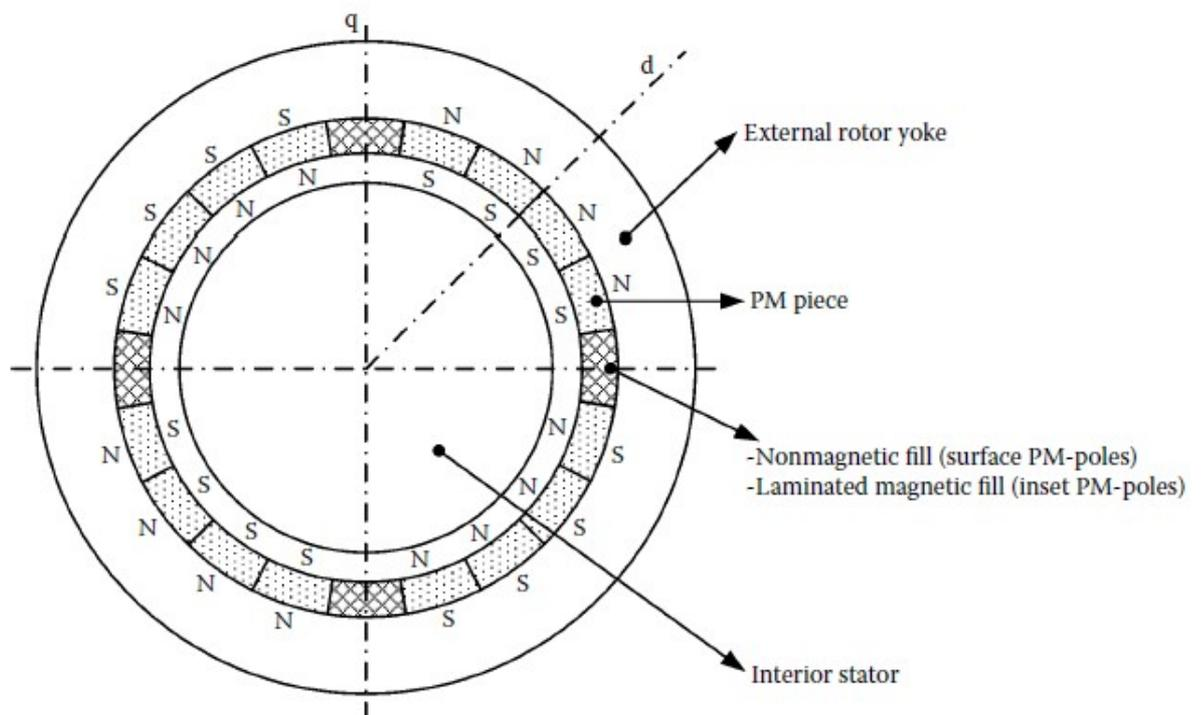
FIGURE Four-pole cylindrical external rotor.
