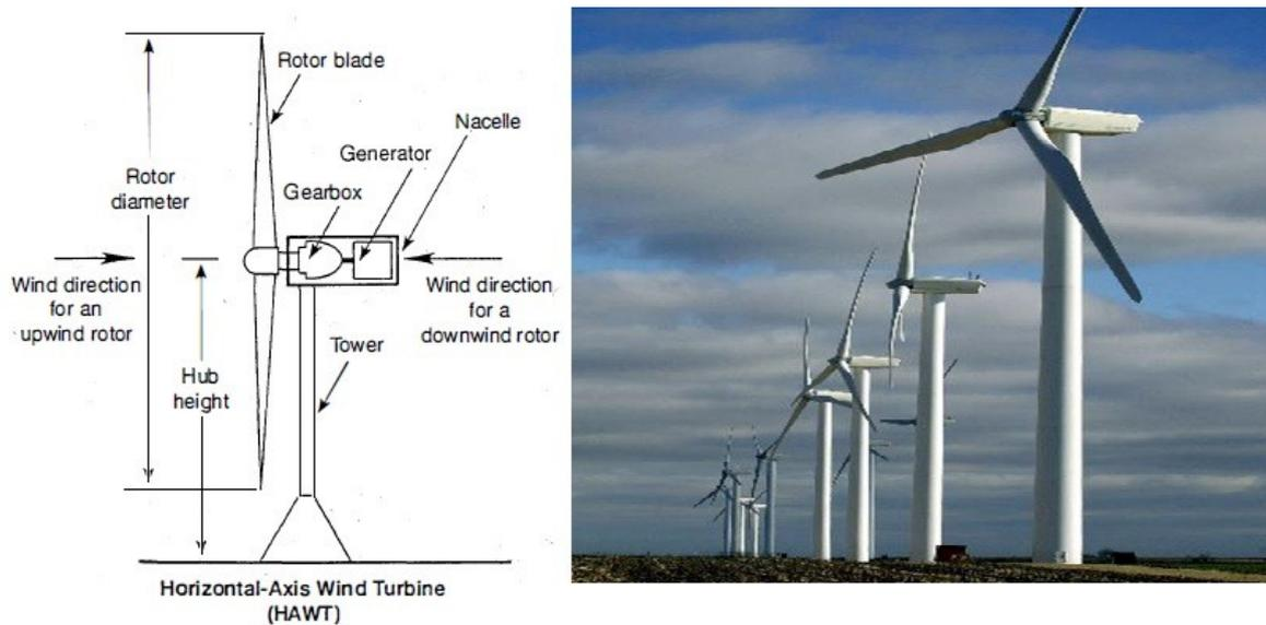
**Figure Horizontal-axis wind turbines**
