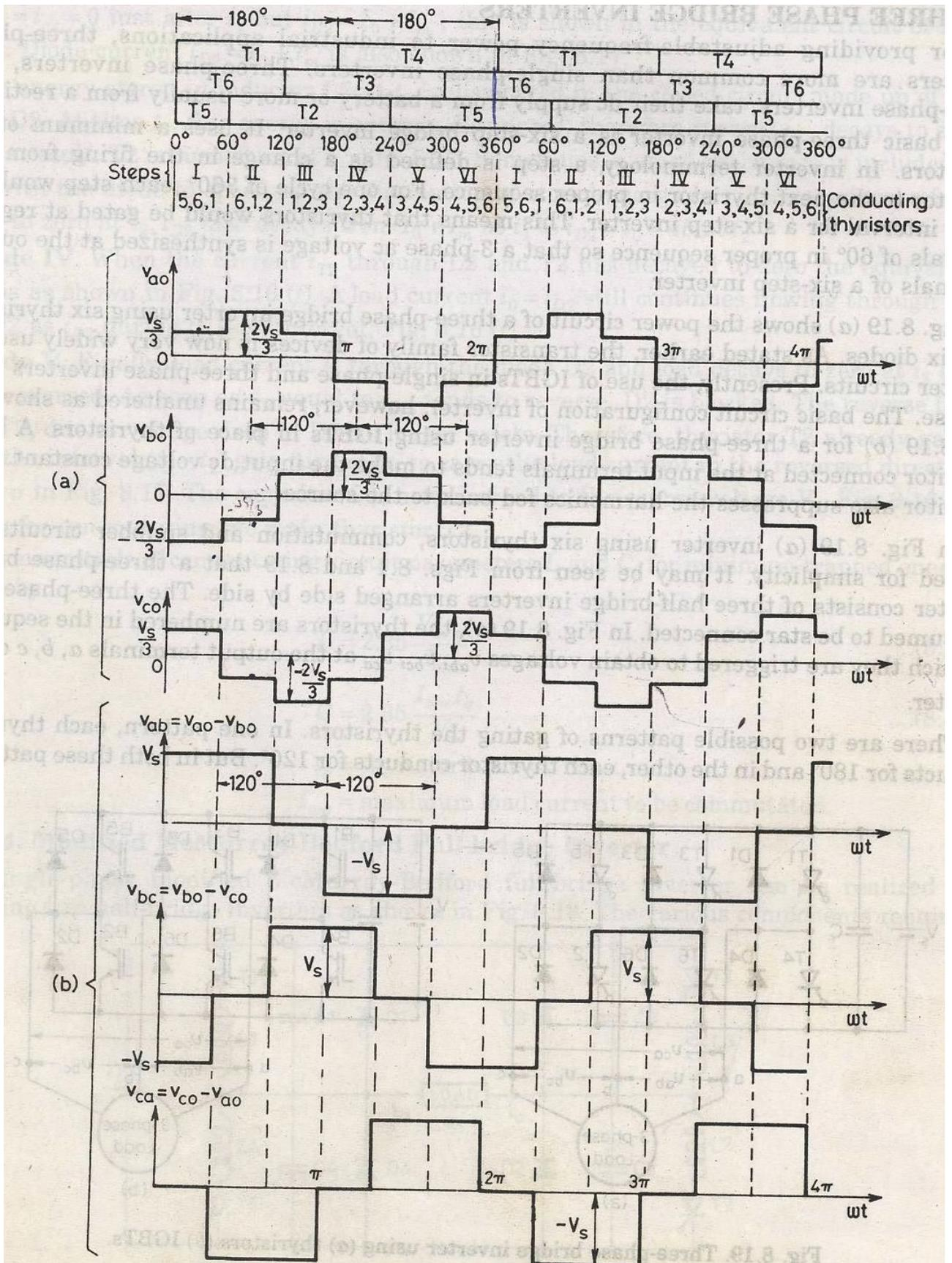
Fig. 8.20. Voltage waveforms for 180° mode 3-phase VSI.
