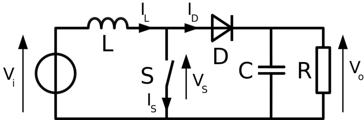
The basic principle of a Boost converter consists of 2 distinct states (see figure below) :
