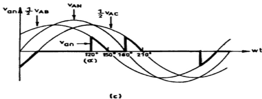
FIGURE Output voltage waveforms for a three-phase ac voltage controller with star-connected  $R$ -load: (a)  $v_{an}$  for  $\alpha = 30^\circ$ ; (b)  $v_{an}$  for  $\alpha = 75^\circ$ ; and (c)  $v_{an}$  for  $\alpha = 120^\circ$ .
