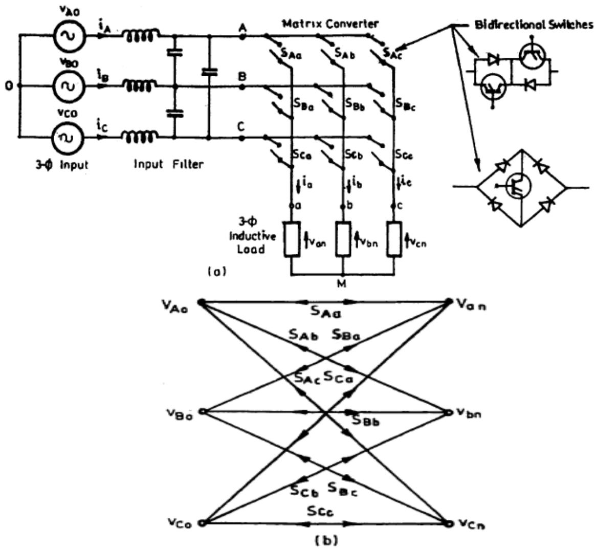
Figure (a) The 3φ-3φ Matrix converter (b) switching matrix symbol for converter
