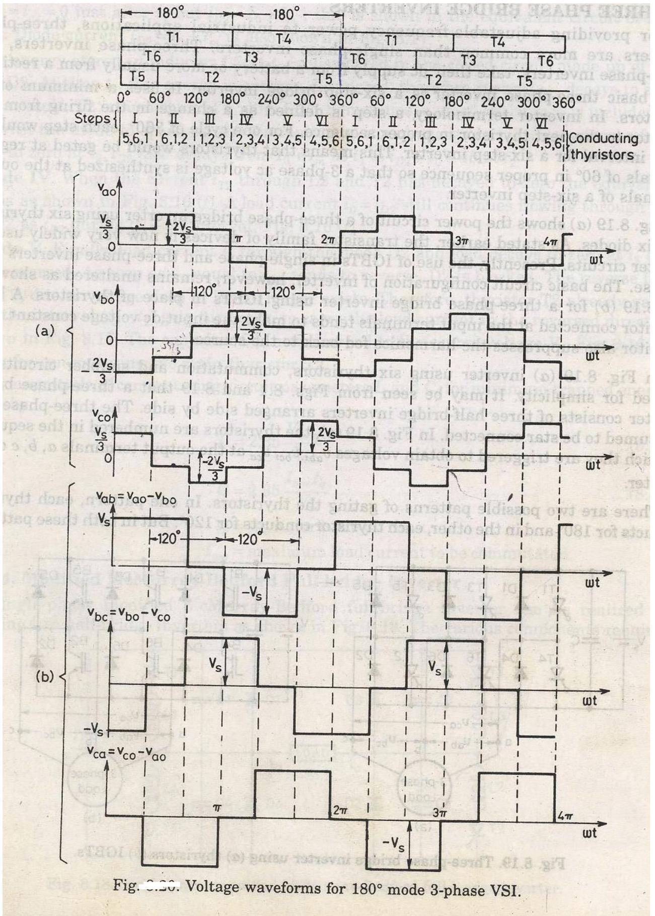
Fig. 8.20. Voltage waveforms for 180° mode 3-phase VSI.
