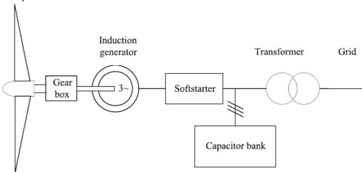
Fig General structure of a fixed-speed WECS
