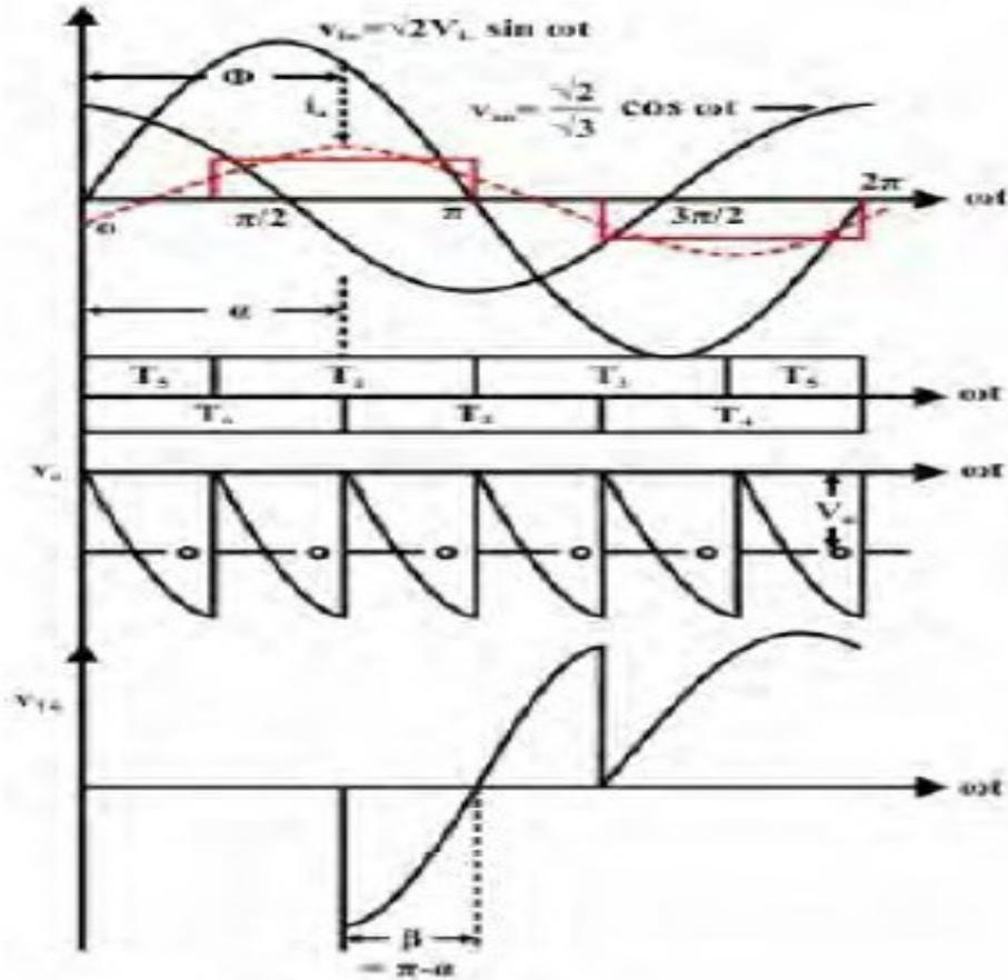
Analysis of the converter in the inverting mode is similar to its rectifier mode of operation. The same expressions hold for the dc and harmonic compounds in the output voltage and current. In particular
