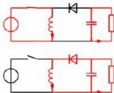
The two operating states of a buck—boost converter: When the switch is turned-on, the input voltage source supplies current to the inductor, and the capacitor supplies current to the resistor (output load).
