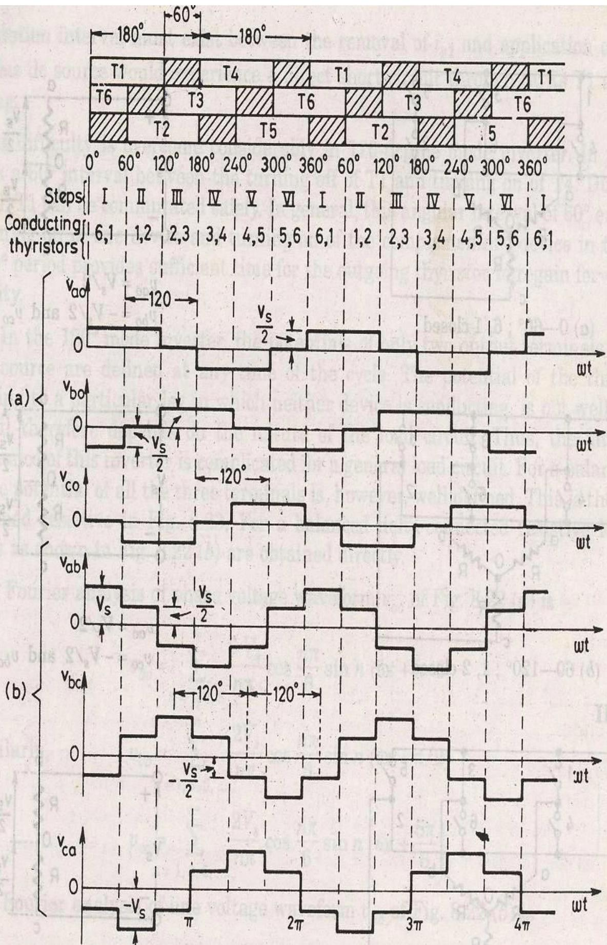
Fig. Voltage waveforms for 120°mode six-step 3-phase VSI.
