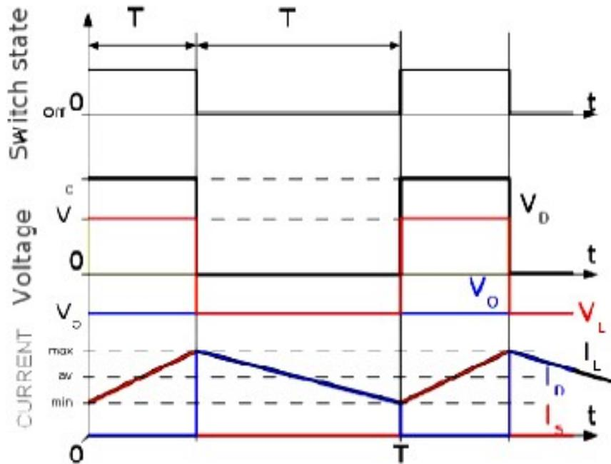
Waveforms of current and voltage in a buck-boost converter operating in continuous mode.
