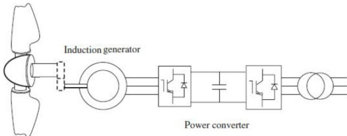
**Figure Typical configuration of a fully rated converter-connected wind turbine**
