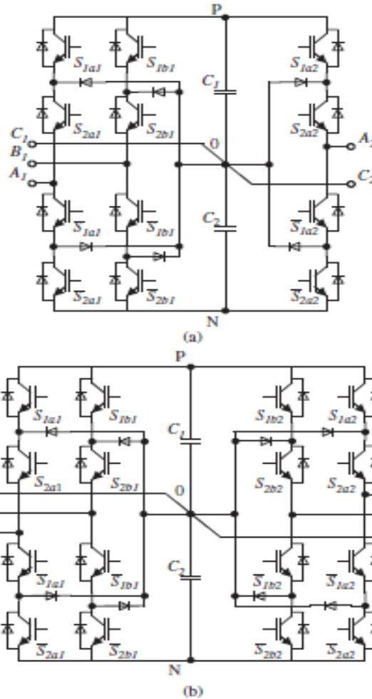
**Figure** Simplified DCC AC–DC–AC converters: (a) three-phase/one-phase (S3L-DCC 3/1) and (b) three-phase/three-phase (S3L-DCC 3/3)
