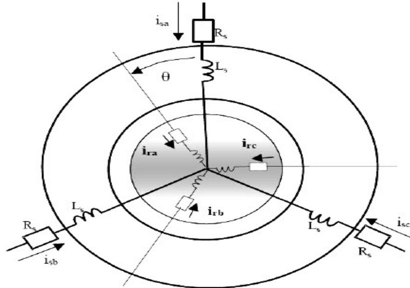
Figure : Induction machine's schematic illustration
