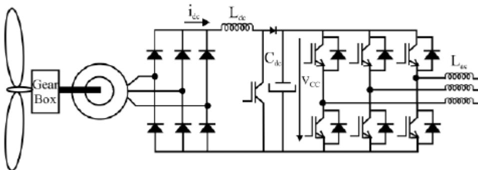
Figure a PMSG with the rectifier, boost chopper, and PWM line-side
