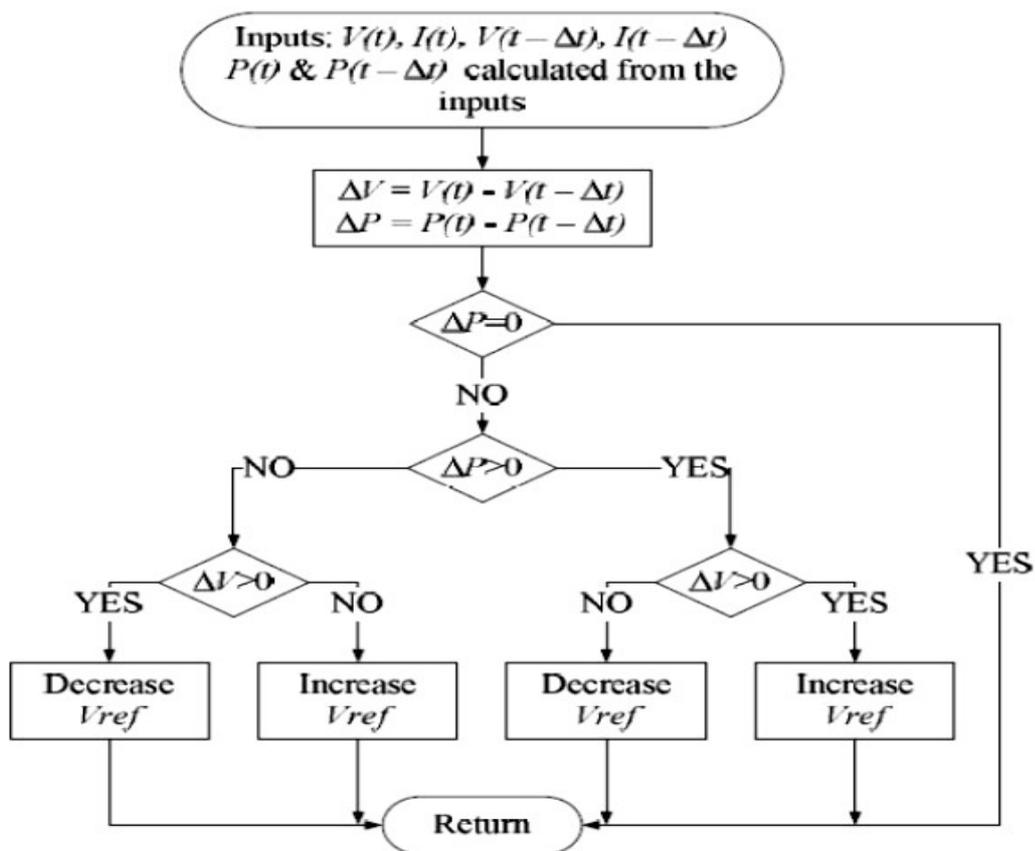
Figure - The flowchart of the P&O Algorithm.
