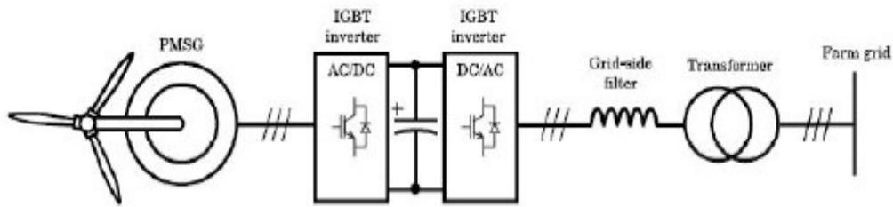
Figure b PMSG with back-to-back PWM converters
